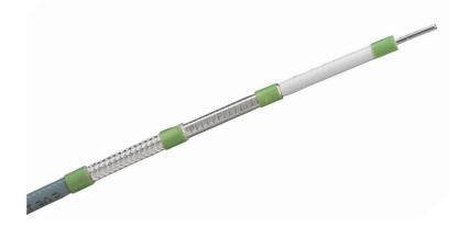
LA190S is a cable design of low loss, high Vp, phase stability and light weight cable for high altitude and space flight applications. The cable is built with ultra low density ePTFE.
